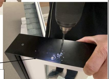
Locate dimple location for hinge holes on opposite end and drill the remaining three hinge holes
