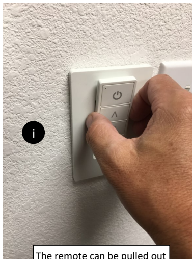
The remote can be pulled out of the wall plate if desired
