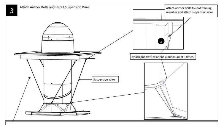
NOTE: It is critical to leave 1 in. (25 mm) of slack in suspension wire for all ICC 500/FEMA P361 applications.
