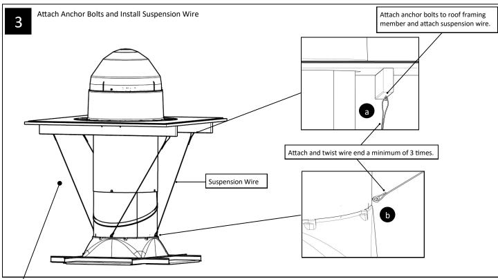
NOTE: It is critical to leave 1 in. (25 mm) of slack in suspension wire for all ICC 500/FEMA P361 applications.
