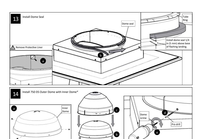
\*Polycarbonate inner dome required for all ICC 500/FEMA P361 applications; dip screw threads in sealant.
