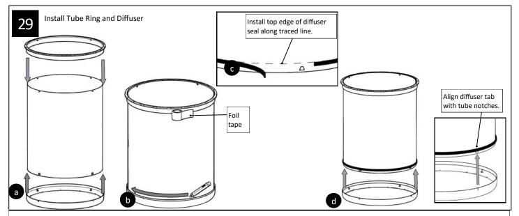
\* For installations where high levels of suit or debris may be present it may be necessary to use foil tape to seal the diffuser to the tubing to prevent the excess debris from entering the tubing.
