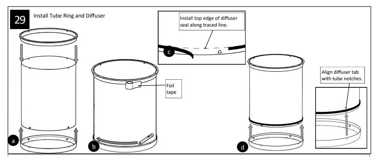
\* For installations where high levels of suit or debris may be present it may be necessary to use foil tape to seal the diffuser to the tubing to prevent the excess debris from entering the tubing.
