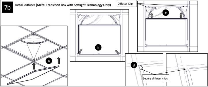
Note: Do not press diffuser into metal transition box too far. Ensure that diffuser is flush with transition box frame.
