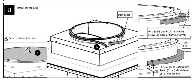
Option 1: Install 330 DS dome 9 Reflective side of LightTracker™ Reflector faces South in Northern Hemisphere (North in Southern Hemisphere). Insert dome spacer long С end first. b Pre-drill d 0-100 LightTracker™ а Reflector tabs fit between Top Tube and Tube Ring. Dome screw е **M** Insert dome screws and spacers evenly leaving every other hole open.
