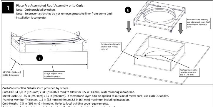
Curb Aspect: Level curb top and plumb curb walls. For sloped roofs add cricket to divert water.
