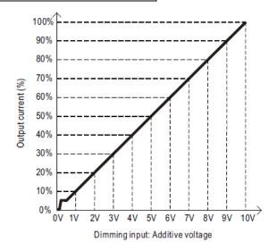
**Note:** The Solatube Integrated LED Light Kit can only be controlled by a sinking controller. If the controller is sourcing the 0-10V signal, the LED light kit will not dim properly.
