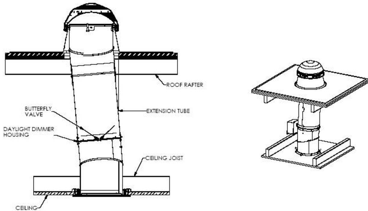
Figure 5 - Typical Solatube Daylight Dimmer Assembly
