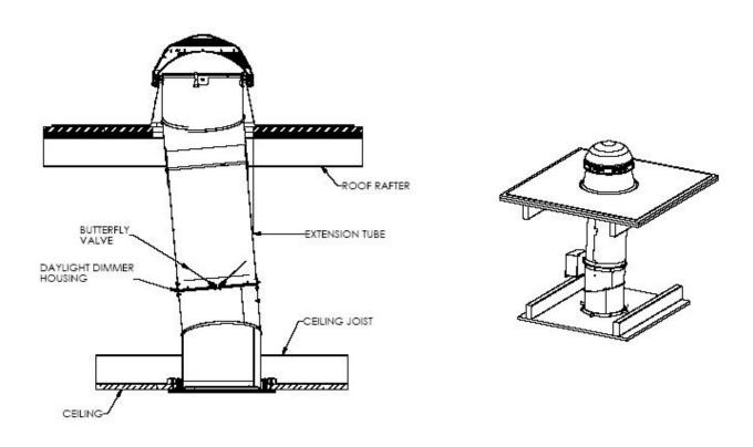
Figure 5 - Typical Solatube Daylight Dimmer Assembly
