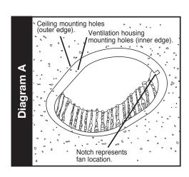
Step 3. For concrete ceilings, use mounting plate as a location guide and mark screw holes. Remove mounting plate and pre-drill outer and inner screw holes. For outer holes, pre-drill hole according to manufacturer recommendations of the fastener used. For inner holes (closest to opening) that are used for attaching Ventilation Housing, the pre-drilled holes need only be approximately ½ inch (12.5 mm) deep (Diagram B).
