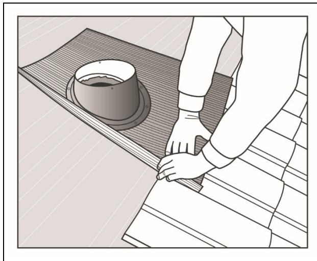
Figure 6 Securing the interlocking tile flashing
