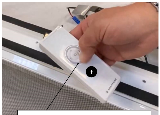
Press the "DOWN" button to bring the chain back to the home position. If motor does not operate, see pairing section on page 21.
