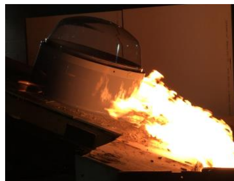
Testing conducted on 330 DS (Polycarbonate Dome) at the FM Global Research Campus in Glocester, RI.
