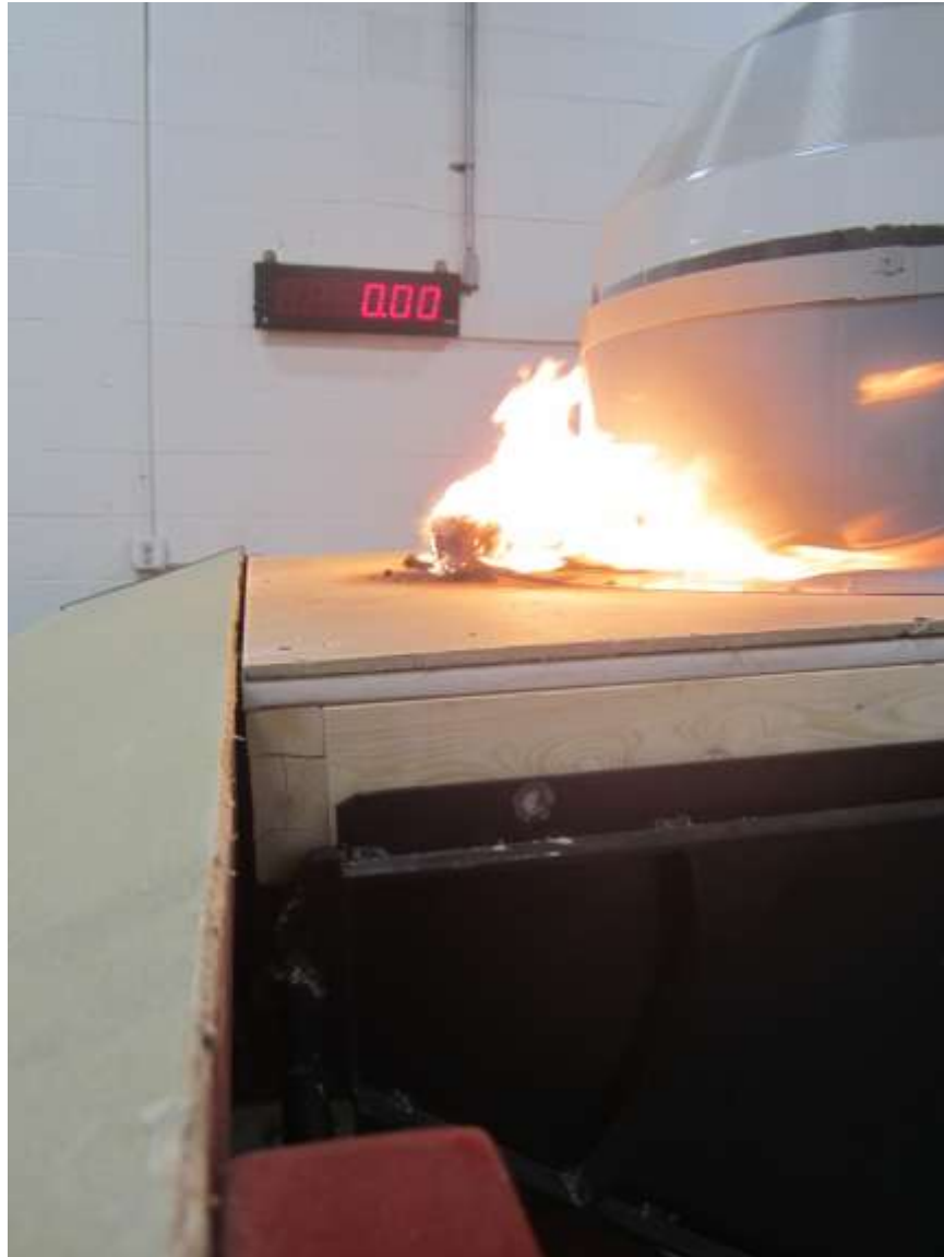
Photo No. 7 Burning Brand Test of 750 DS
