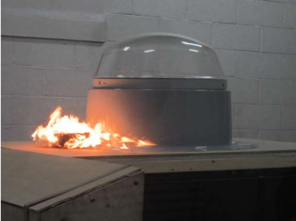
Photo No. 3 Burning Brand Test of 330 DS
